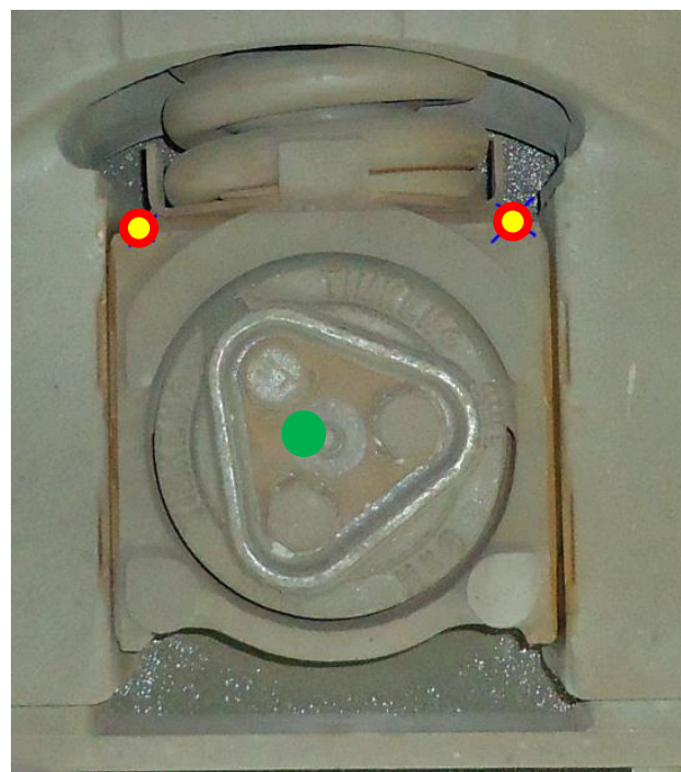
Figure 11 : Outside view: green: temperature measurement (use bolt to fix the system or use thermocouple gauge directly glued on the surface...)
