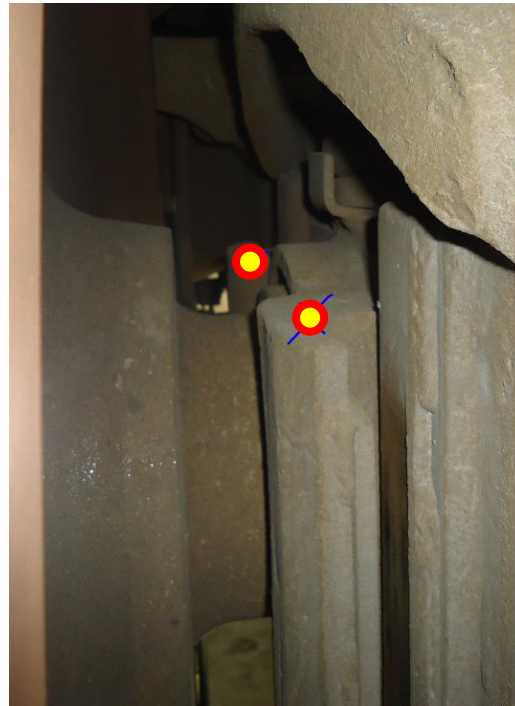
Figure 10 : On wheel side: preferred (protected and in the wagon gauge)
