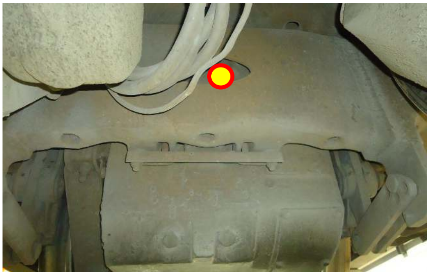
Figure 6 : IMU suggested location: flat, easy access, centre of bogie, protected...
