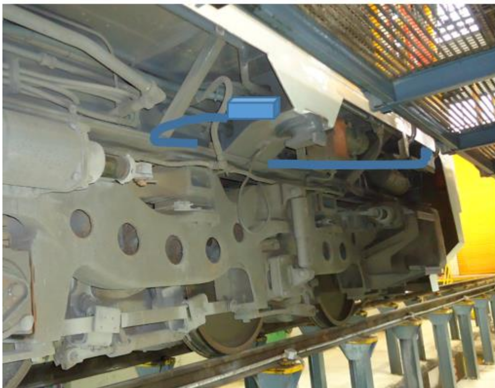
Figure 3 : Available position on outside part of the cabin to put the conditioning system
