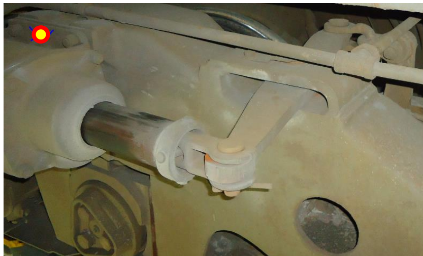
Figure 9 : Close-up view of accelerometer position (behind the hydraulic system of the brake = protected area)
