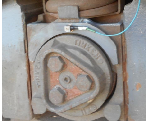
Figure 9 : High frequency tri axial accelerometer (PCB 356A02) on an axle box
